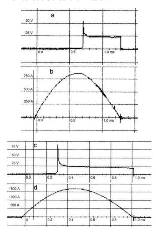
Fig. 5 Current and arcing voltage traces of an ultra short fuse for two different prospective currents: the silver fuse element, 1 mm long with the cross-sectional area of 0,07 mm<sup>2</sup>
