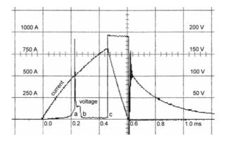
Fig. 2 CHCL operation: a – fuse arc ignition, b – transistor on, c – transistor off
