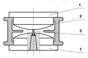
Fig. 6 Example design of an ultra-short fuse
