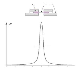
Fig. 4. Temperature distribution along the short fuse: 1 – the fuse element, 2 – terminal, 3 – solder, 2-mm horizontal division
