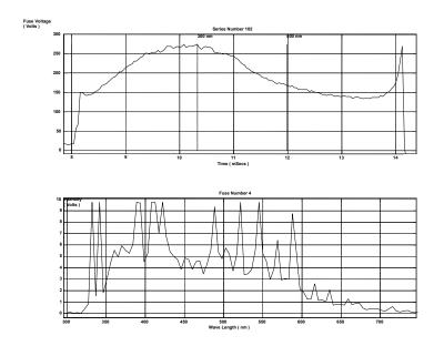
Figure 7 Typical arc light spectrum and correlated fuse voltage oscillogram captured during the post-peak arc voltage time period of disintegration in a short notch silver element fuse
