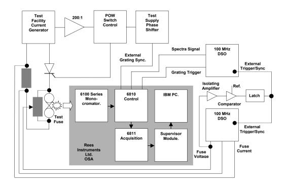
Figure 2 Diagram of optical spectrum analyser interfaced to the fuse test facility
