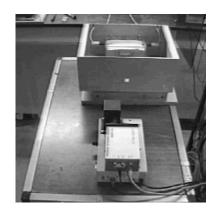
Figure 4 Experimental arrangement of OSA and fuse enclosure (Shown without top cover and opaque shroud)
