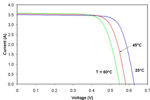
**Fig. 1:** I-V Characteristic for PV cell
