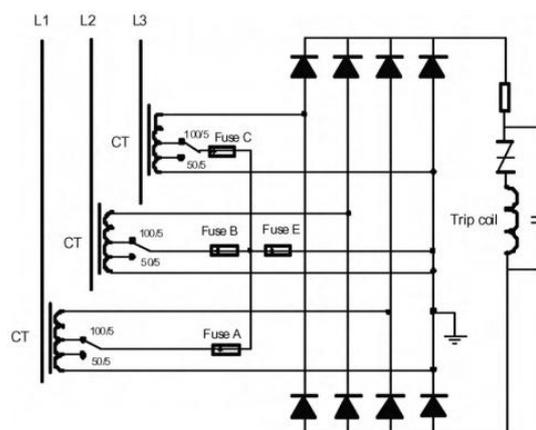
**Fig. 4.3:** New protection system based on the TLF (Time Limite Fuse).
