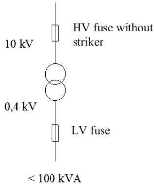
Fig. 2.1: Protection with fuses on the high-voltage and low-voltage sides.
