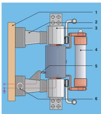
**Fig. 4.2:** Base and link of  $I_s$  limiter; 1-base plate, 2-insulator, 3-head pole with clamp, 4-fuse, 5-telescopic contact, 6-insulator with pulse transformer.
