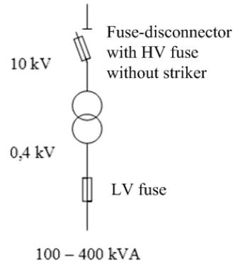
Fig. 2.3: Protection with fuse-disconnector on the HV side, and with fuses on the LV side.
