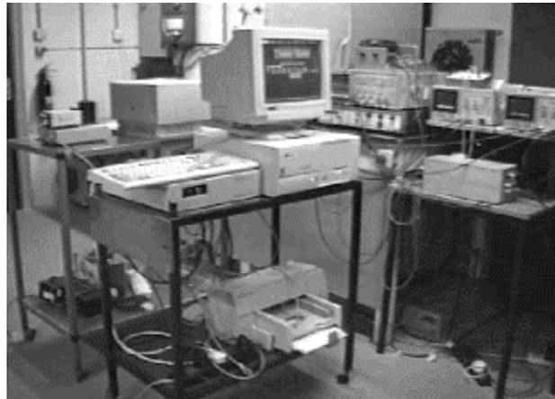
Figure 3 Experimental arrangement used in the spectroscopic analysis of HBC conductive film substrate fuse arcing phenomena.
