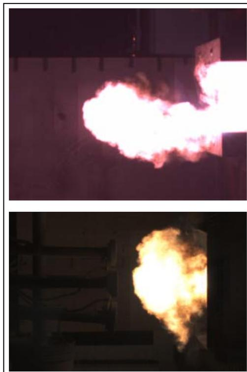
Fig. 5: Side view of arc development from barrier tests 4ms into a 42kA, 480V event. Open configuration (Top) and in a enclosure (Bottom).
