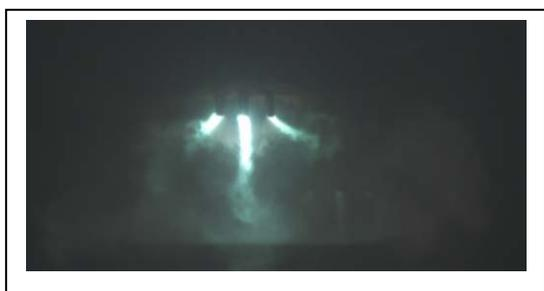
Fig. 3: Front view of arc development from vertical test 3ms into event.
