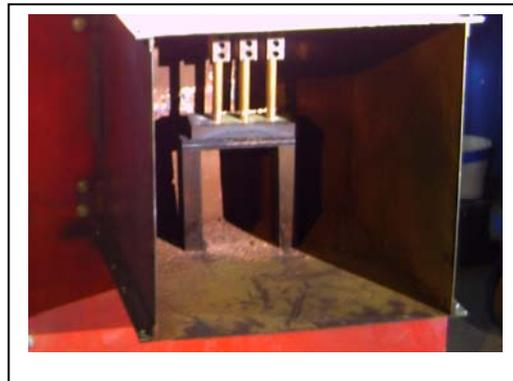
Fig. 4: Barrier test configuration simulating the line side connections of top fed equipment.
