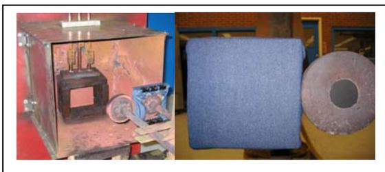
Fig. 9: Fabric test setup with barrier test (Left); Front view of bare and fabric covered calorimeter (Right)
