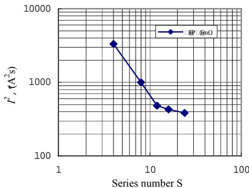
Fig. 9: S -  $I^2t$  characteristics (for the 8P series).
