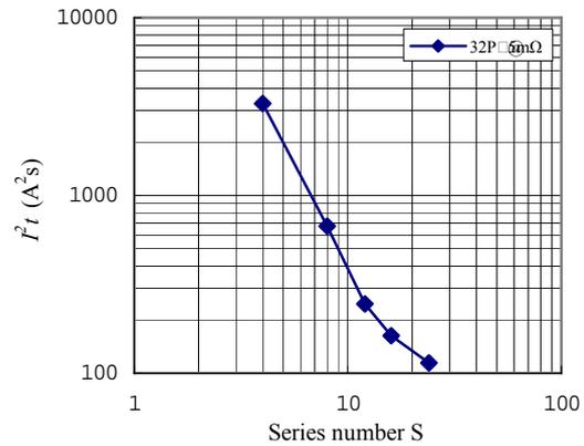
Fig. 10: S -  $I^2t$  characteristics (for the 32P series).
