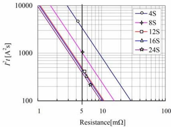
Fig. 8: Resistance -  $I^2t$  characteristics (8P series).
