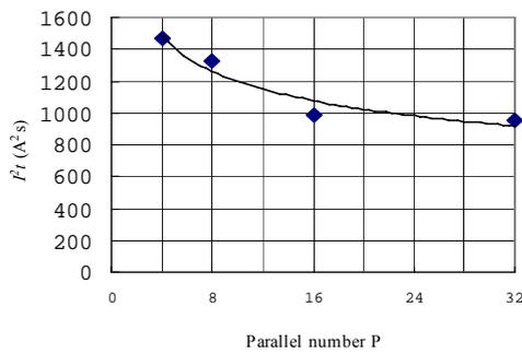
Fig. 6: Parallel number  $P$  -  $I^2t$  characteristic (6S series).
