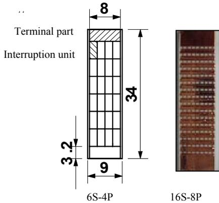
Fig. 2: Fuse structure (units in mm).
