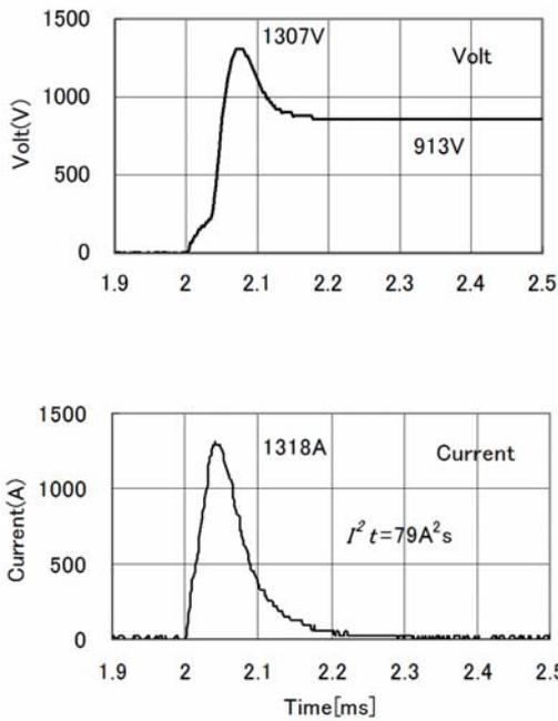
Fig. 5: Oscillograms of interruption tests of 24S-32P.
