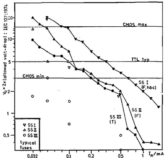
Fig. 1  $I_n$  : Minimum operating voltage at twice IEC127 voltage-drop limits.
