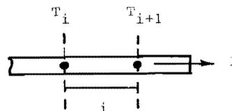
Fig.1 Division of wire element into finite sections.
