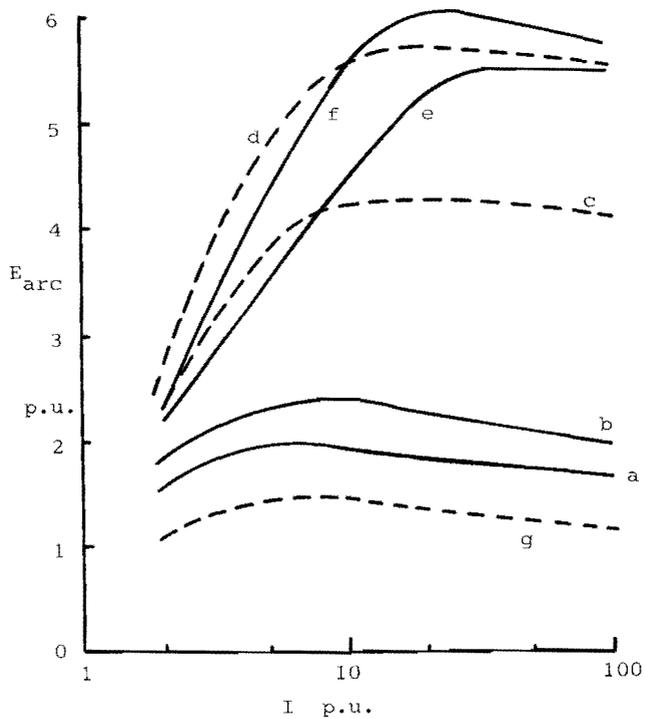
Fig.6 Arc energy characteristics for fuse HV.
