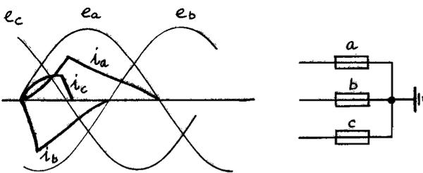
Fig.2 Fault current transients. (Earthed,  $\theta = 0^\circ$ )
