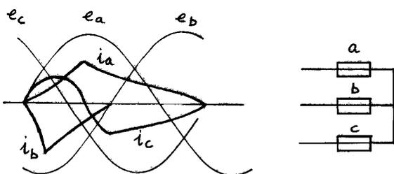
Fig.3 Fault current transients. (Unearthed,  $\theta = 0^\circ$ )
