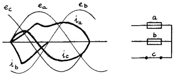
Fig.4 Fault current transients. (2 fuses, unearthed,  $\theta = 0^\circ$ )
