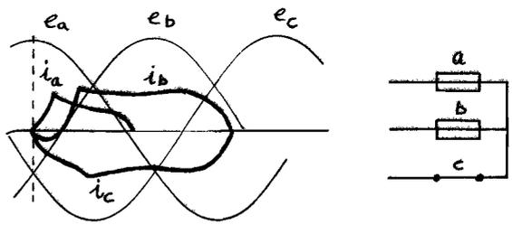
Fig.5 Fault current transients. (2 fuses, unearthed,  $\theta = 90^\circ$ )
